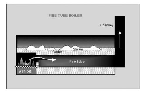
Figure: Sectional view of a fire tube boiler *Reference: http://www.bathtram.org/tfb/tT111.htm*
