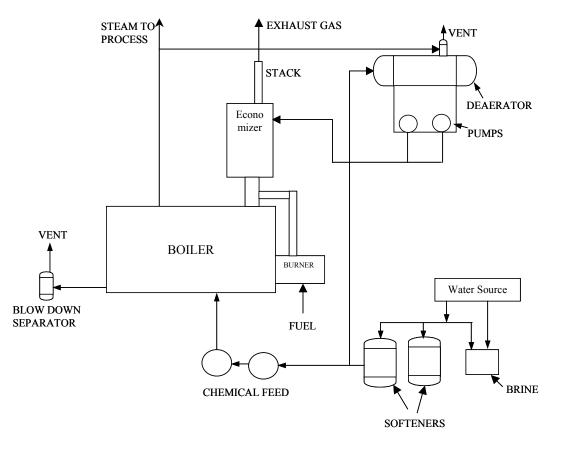
Figure: A typical schematic of a boiler room Reference: National Productivity Council
