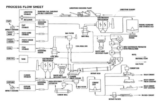
Figure 1: Cement Production Process. *Reference: http://www.acclimited.com*
