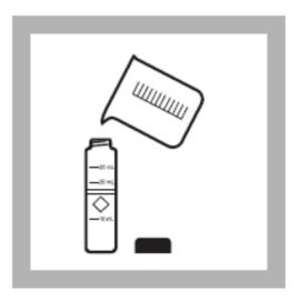
**4.** Fill a second sample cell with 10 mL of the sample.
