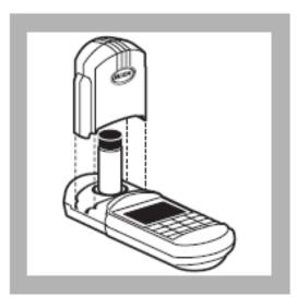
**9.** After the timer beeps, place the prepared sample into the cell holder. Tightly cover the sample cell with the instrument cap.
