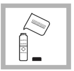
**3.** Fill a sample cell with 10 mL of sample.
