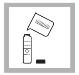
**6.** Fill another sample cell with 10 mL of sample (the blank).
