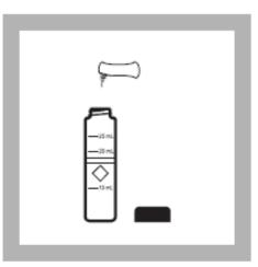
4. Add the contents of one PhosVer 3 Phosphate Powder Pillow for 10-mL sample to the cell (the prepared sample). Shake for 15 seconds.
