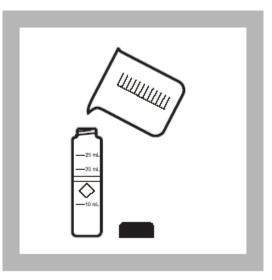
8. Stir the sample thoroughly and immediately pour 25 mL of the blended sample into a sample cell (the prepared sample).
