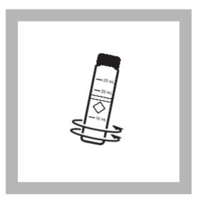
**9.** Swirl the prepared sample cell to remove any gas bubbles and uniformly suspend any residue.
