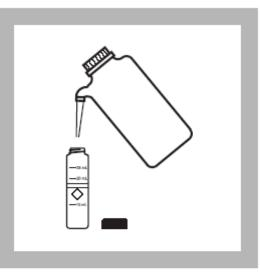
**5.** Fill a sample cell with 25 mL of tap water or deionized water (the blank).
