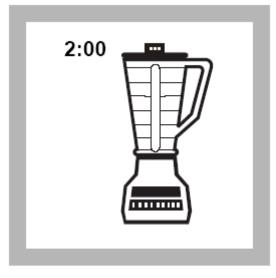
Blend 500 mL of sample in a blender at high speed for exactly 2 minutes.
