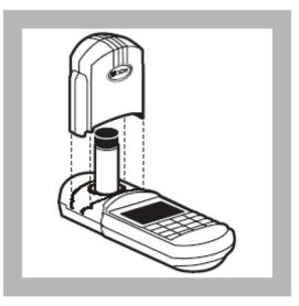
**10.** Place the prepared sample into the cell holder. Tightly cover the sample cell with the instrument cap.
