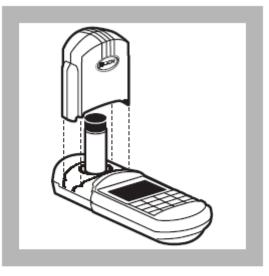
**6.** Place the blank in the cell holder. Tightly cover the sample cell with the instrument cap.
