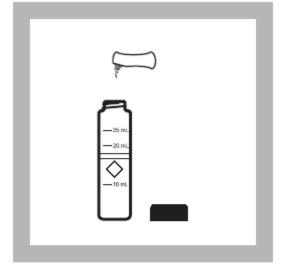
4. Add the contents of one ZincoVer 5 Reagent Powder Pillow. Cap. Invert several times to completely dissolve the powder. If the sample does not turn orange, see the note below.
