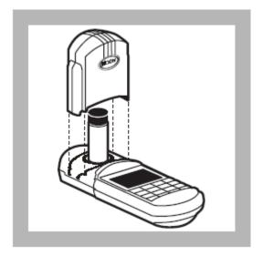
11. Immediately place the prepared sample into the cell holder. Tightly cover the sample cell with the instrument cap.
