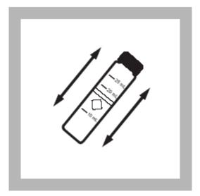
7. Tightly cap the cell. Shake vigorously for 30 seconds (the prepared sample).
