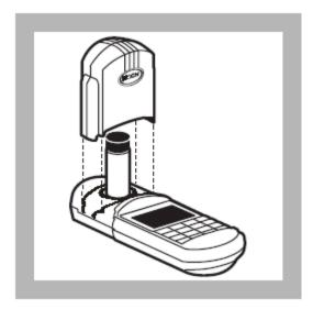
**9.** Place the blank into the cell holder. Tightly cover the sample cell with the instrument cap.
