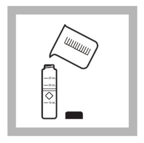
**3.** Fill a 25-mL sample cell with 20 mL of sample.
