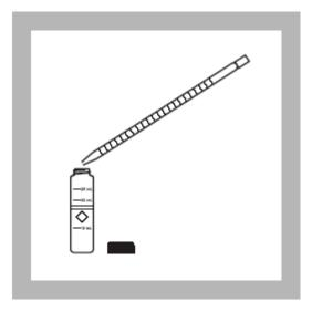
**5.** Measure 10 mL of the orange solution into another sample cell (the blank).
