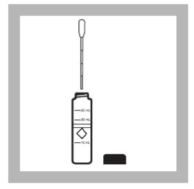
**6.** Add 0.5 mL of cyclohexanone to the remaining orange solution in the first sample cell (the prepared sample).
