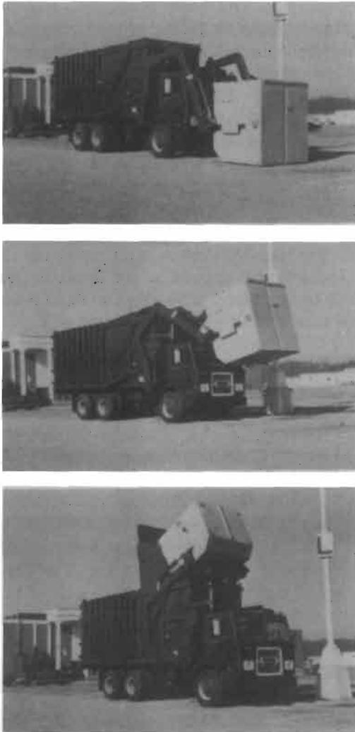
**Figure 12-2.** Containerized collection system. (Courtesy of Dempster Systems.)
