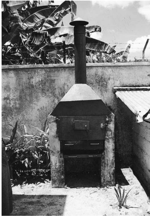
*Fig. 8.3 Single-chamber incinerator*
