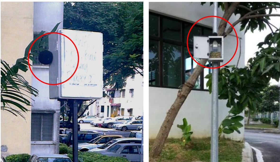
**Figure B-15: Examples of unacceptable use of sound level meter installed in a casing as an alternative to permanent noise monitoring units**
