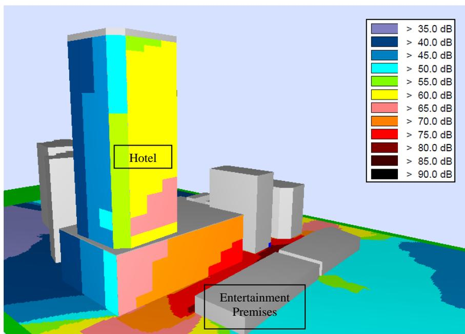
**Figure 11: Noise propagation from 3-D noise modelling of entertainment noise sources from a row of entertainment premises affecting adjacent sensitive receptors**
