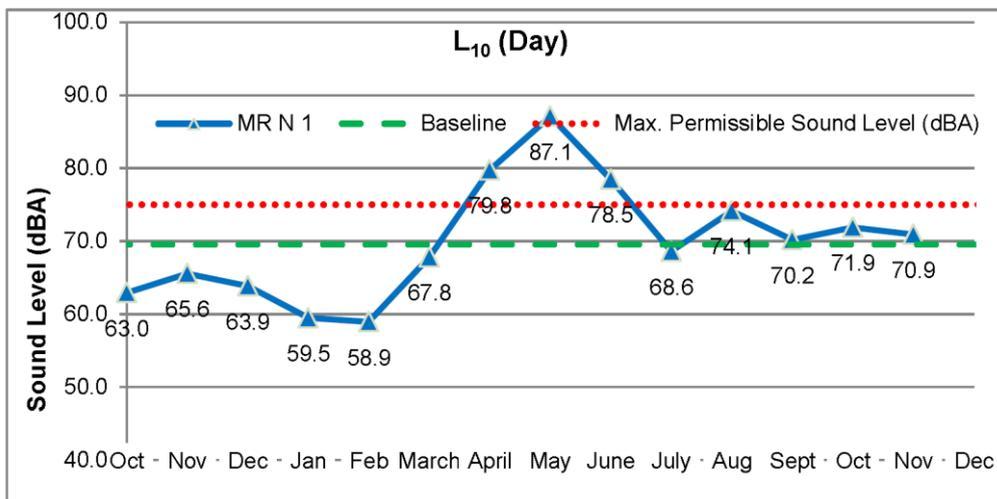
**Figure B-37: Example of trending of noise measurements results (Daytime L<sub>10</sub> levels) over one year assessed against permissible and baseline levels**
