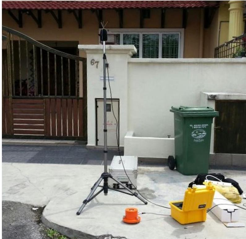
**Figure B-1: Example of sound level meter for environmental noise measurements**
