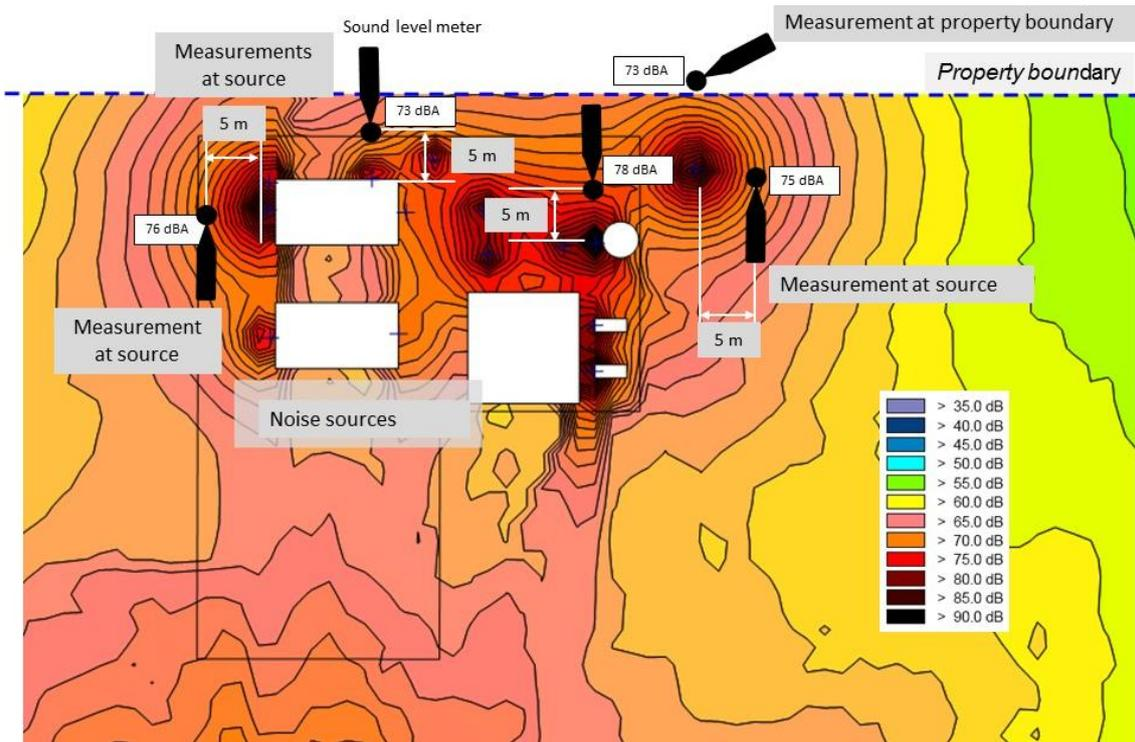
**Figure B-10:** Example of noise source measurement in industrial plants
