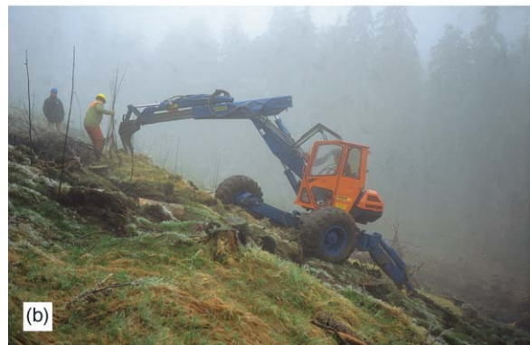
Figure 19 (a) Various modern planting hoes; (b) modern sapling planting machine.
