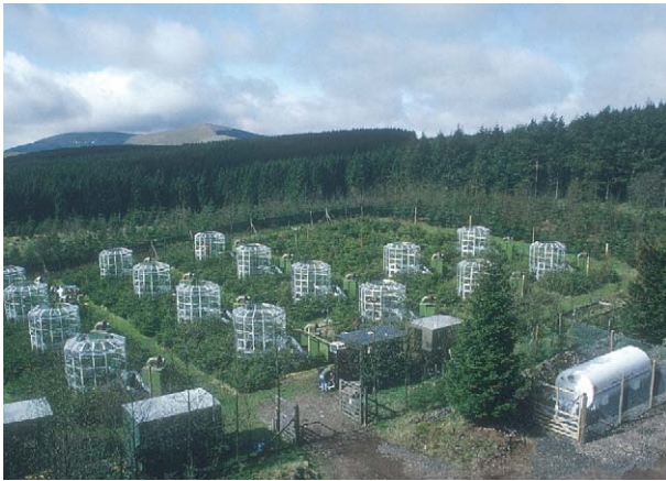
Figure 3 Open top chambers (OTCs) at Glendevon, Perthshire, Scotland. Half of the chambers are flushed with ambient air and half with ambient air with additional CO 2 added to maintain a CO 2 concentration of twice ambient. The CO 2 tank can be seen in the foreground. The control room is just inside the site gates, and a nonchamber control area containing four plots with trees but no chambers can be seen at the rear, right of the photograph. This area was included to assess the effects of the chambers themselves on the trees. Photograph courtesy of the Forest Research Photo Library.
