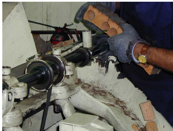
Figure 10 Boring of stoppers from a cork strip in the industry.
