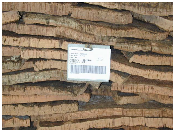
Figure 9 Cork planks after the water-boiling operation.
