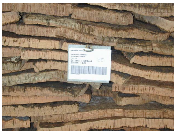
Figure 9 Cork planks after the water-boiling operation.
