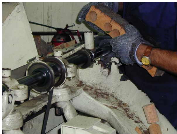
Figure 10 Boring of stoppers from a cork strip in the industry.
