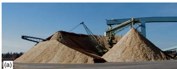
Figure 16 The sawmill or satellite woodyard screen system (a) with only a gyratory screen is much less complex than a thickness screening system installed in most woodyards (b). Note the aerodynamic separator up-draft tubes can be seen on the closest side of the system.
