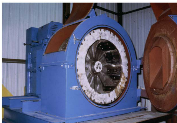
Figure 13 Chip slicing. The two rings in the slicer rotate in the same direction, but the inside ring brings the chips to the knife at a faster speed than the knife ring is rotating.
