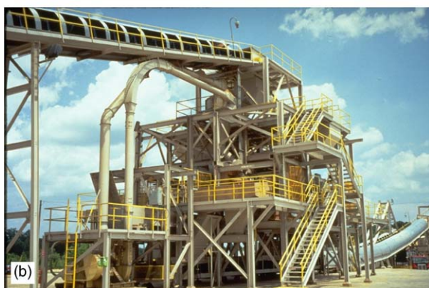
Figure 16 The sawmill or satellite woodyard screen system (a) with only a gyratory screen is much less complex than a thickness screening system installed in most woodyards (b). Note the aerodynamic separator up-draft tubes can be seen on the closest side of the system.
