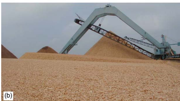
Figure 18 State-of-the-art chip storage systems. Automated outstocking and reclaim is used to maintain a first-in/first-out pile rotation. The arrangement is either circular (a) or linear (b).
