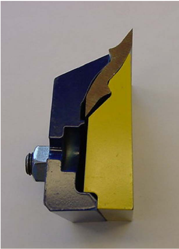
Figure 10 A cut-away section of a disposable chipper knife clamped into a knife holder that is then bolted into the knife pocket. Note the two chipping surfaces that allow the knife to be turned over when one side becomes dull.
