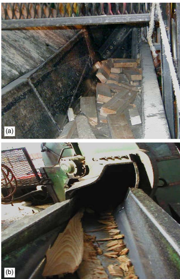
Figure 5 Sawmill chipper infeed. Vibratory conveyors are commonly used to convey sawmill waste to chippers. The size and shape of sawmill by-products varies widely. Some flows are relatively uniform (a) while others contain long slabs, trim blocks, and chip screen oversize (b). uniform sawmill chipper feed material produces more uniform chips.
