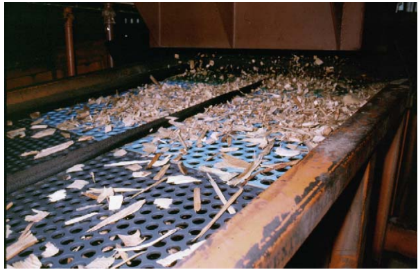
Figure 12 A typical gyratory screen. Note that the round holes are larger in the feed end of the screen and smaller at the discharge end. This has been used to increase screen capacity, but actually reduces removal efficiency.
