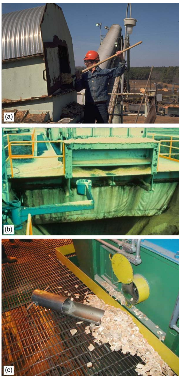
Figure 21 Options for chip sampling. (a) Manual sampling at a belt transfer point using a scoop sized to collect enough chips for the tests being done; (b) an automatic sampler using a bucket mounted on a swinging arm for truck dump sampling; (c) a tube sampler and sample port at a chip screen system to remove chips after screening.
