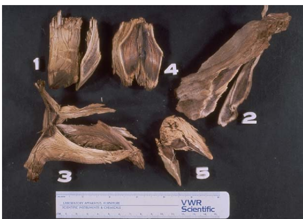
Figure 17 Oversize chips after kraft pulping. (1) Overthick chip with partial impregnation and a woody center; (2) overlength and over thick chip with only the first few millimeters on the outside that are pulped; (3) the distorted grain and compression wood near a branch created an oversize that has only surface pulping; (4) an over thick chip with a woody center; (5) knotwood creates a badly formed chip that only pulps on the surface.
