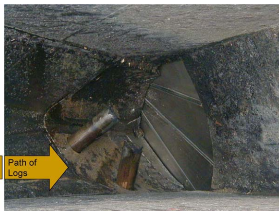
Figure 25 Rams that can be pushed into the chipper infeed to dislodge logs that sometimes frequently plug the spout. This is much safer than trying to break up the jam with pike poles or log tongs and takes less time.
