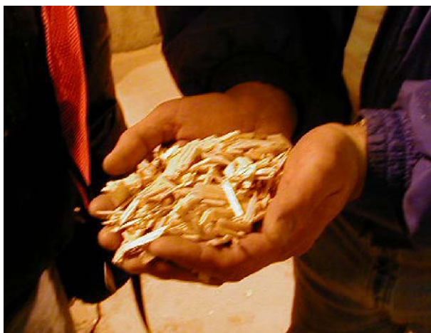
Figure 1 Typical pulp chips sampled after going through the chip screen system.
