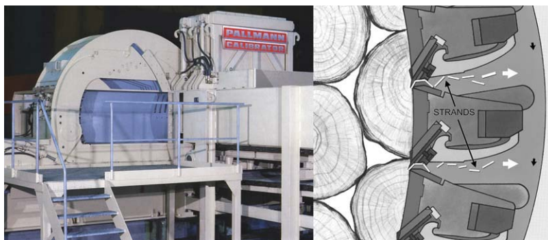
Figure 5 Long-log knife-ring flaker for producing strands for OSB and laminated strand lumber. Cutting action of the knives is shown at right. Photograph courtesy of Pallmann Pulverizers Co., Inc.
