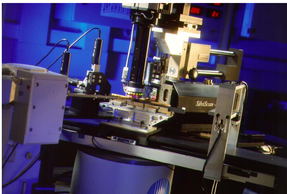
Figure 3 The SilviScan ® instrument combines X-ray densitometry, diffractometry and image analysis to measure a variety of properties in a single wood sample. Photograph courtesy of CSIRO.
