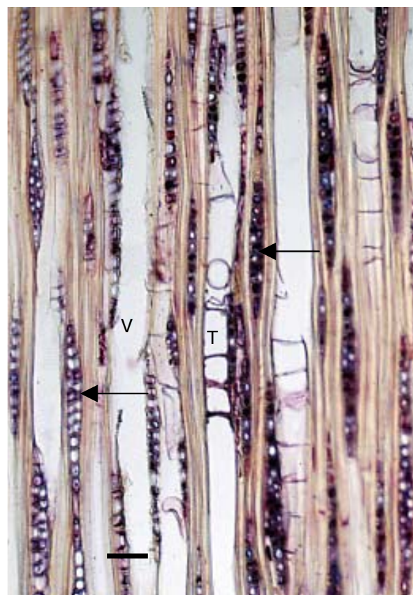
Figure 4 Tangential longitudinal section through wood of Liquidambar styraciflua . The cut ends of rays are seen interspersed among the fibers and vessels (arrows). The vessels (V) contain some tyloses (T). Scale bar = 100 \mu m.
