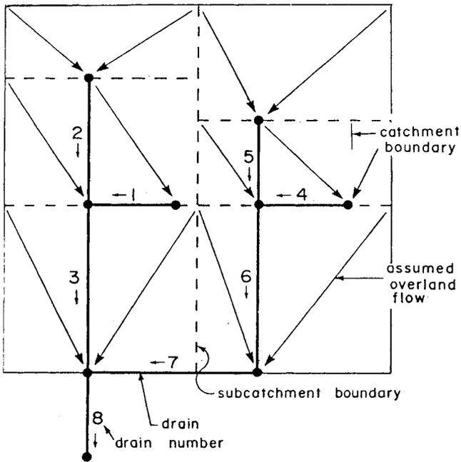
Fig. 5.13 Layout plan of drainage network sized in example.
