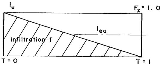
Fig. 5.2 Rectangular hyetograph with decaying losses resulting in triangular excess rain distribution with time
