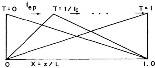
Fig. 5.8 Storm travelling along basin
