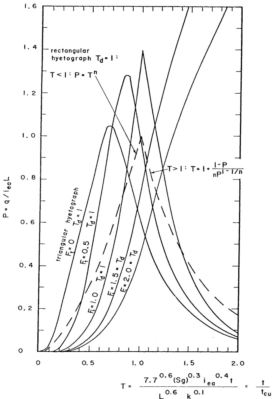
Fig. 5.3: Runoff hydrographs for triangular storm time distribution.  $F_t = t_p / t_c$  where  $t_p$  = time to peak of excess rain and storm duration  $t_d = t_c$  = concentration time for rectangular storm input except for  $F > 1$
