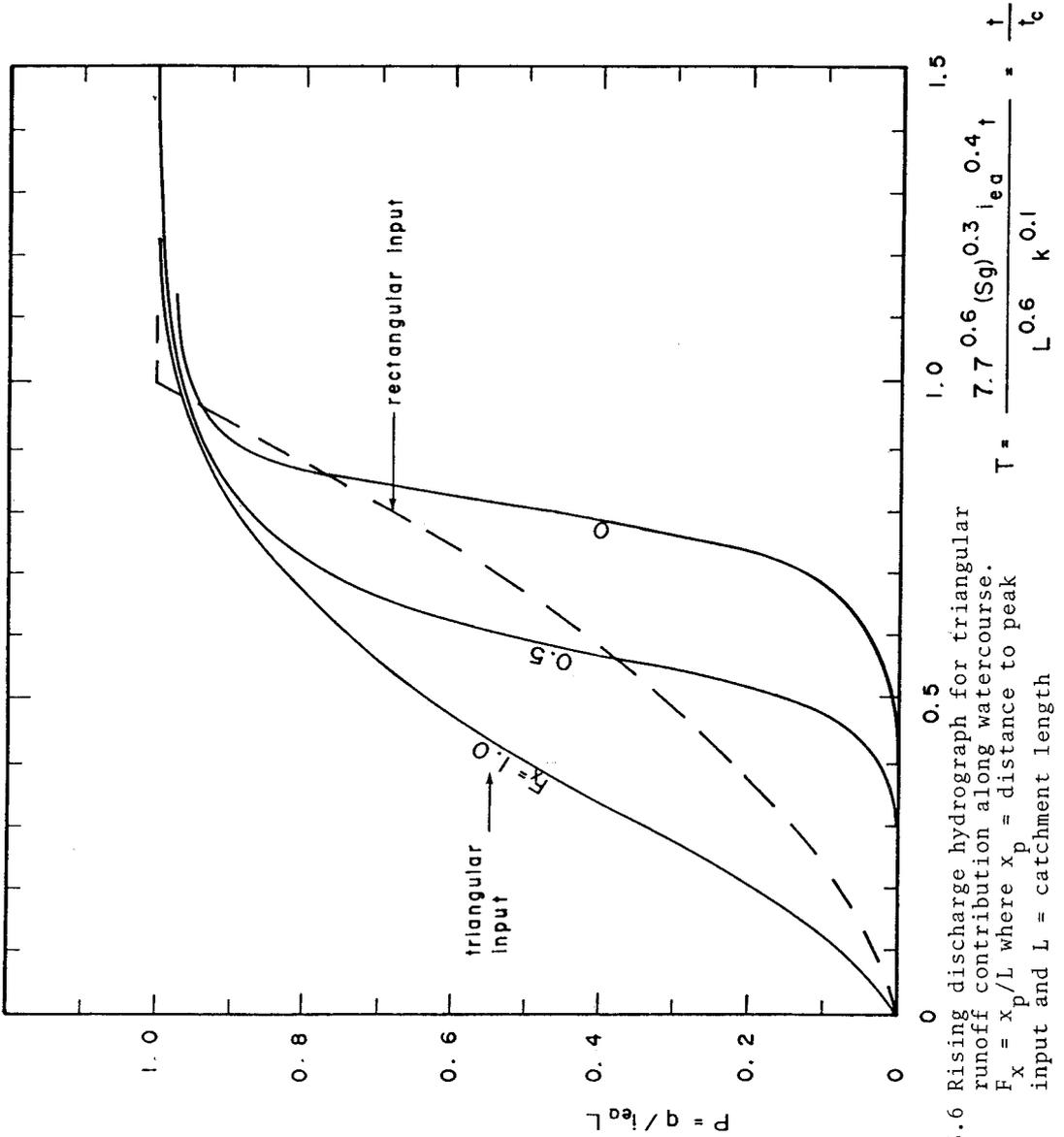
Fig. 5.6 Rising discharge hydrograph for triangular runoff contribution along watercourse.
