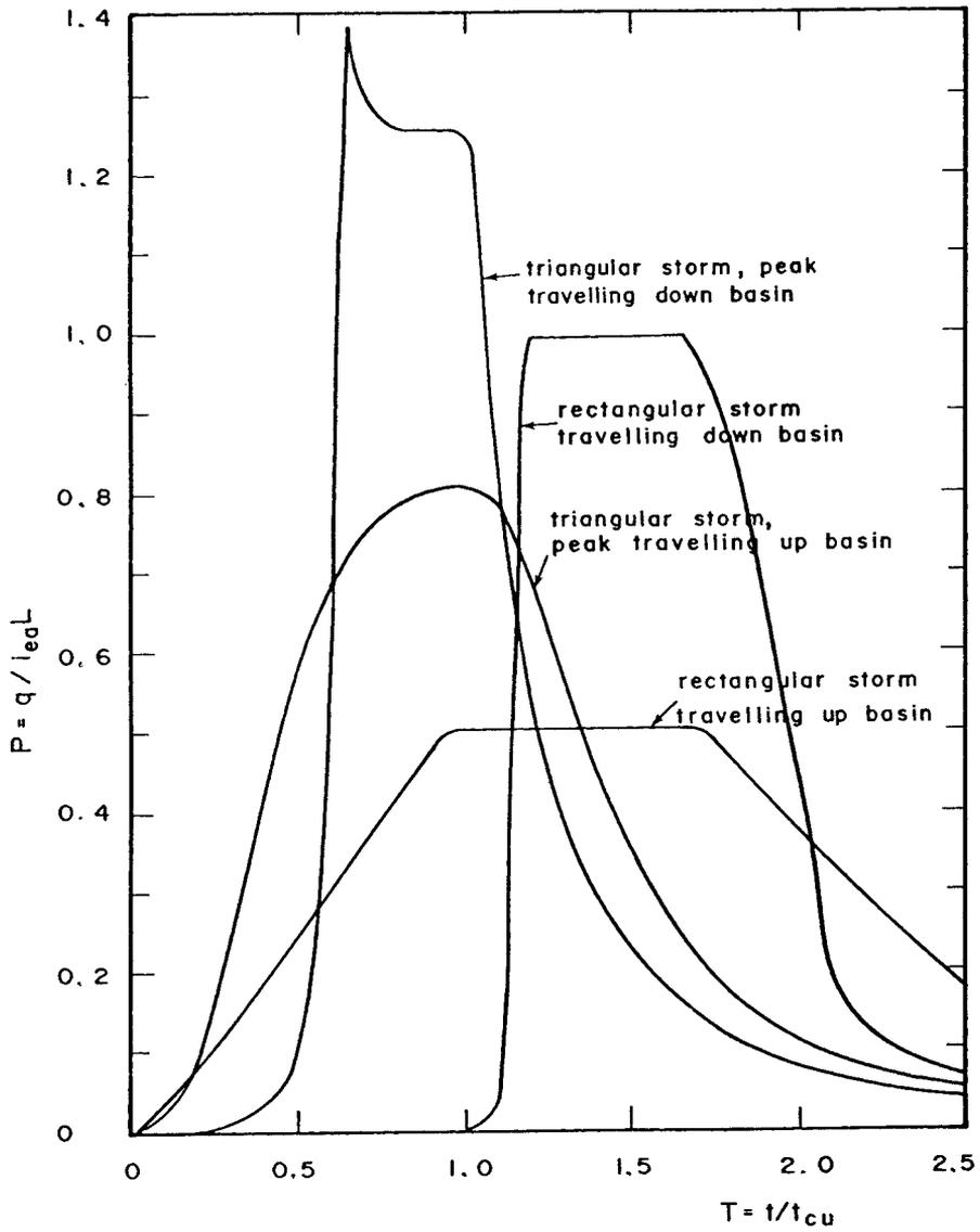
Fig. 5.9 Discharge hydrographs due to travelling storm of duration  $t_c$
