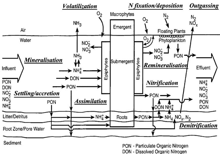
Figure 1: Key nitrogen transformations in SF treatment wetlands (USEPA, 2000).  $\text{NO}_x$  refers to  $\text{NO}_2$  and  $\text{NO}_3$ -N; PON and DON refer to particulate and dissolved organic forms of N (Org-N).
