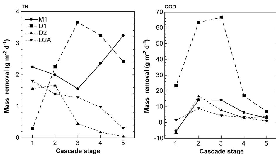
Figure 5: Gradients of TN and COD mass removal during passage through cascade mesocosms simulating horizontal-flow SSF constructed wetlands for four agricultural wastewaters with differing N species balances (Tanner and Kadlec, 2003). The wastewaters had been pretreated in waste stabilisation ponds; M1 = anaerobic-treated meat processing, D1, D2, D2A = anaerobic, facultative and aerated pond treated farm dairy, respectively. See Tanner et al. (2002) for gradients of different N forms.
