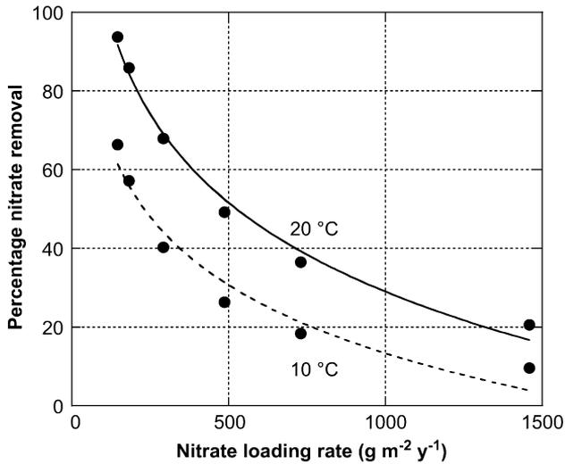
Figure 9: Theoretical relationship between wetland nitrate removal efficiency and loading at 10 and 20°C, based on  $k$ -C \* tanks-in-series kinetic model (IWA, 2000; Kadlec, 2004) with first order areal annual rate constant  $K_{20} = 34$ , temperature factor  $\theta = 1.09$ , hydraulic efficiency parameter  $N = 3$ , influent  $\text{NO}_3\text{-N} = 10 \text{ g m}^{-3}$ , and areal hydraulic loading rate 40–400  $\text{mm day}^{-1}$ .
