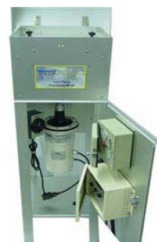
High Volume Air Sampler (HVAS)
