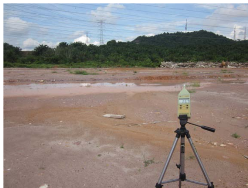
Figure 4.22: Calibrated sound level meter Model: Lutron SL -4001
