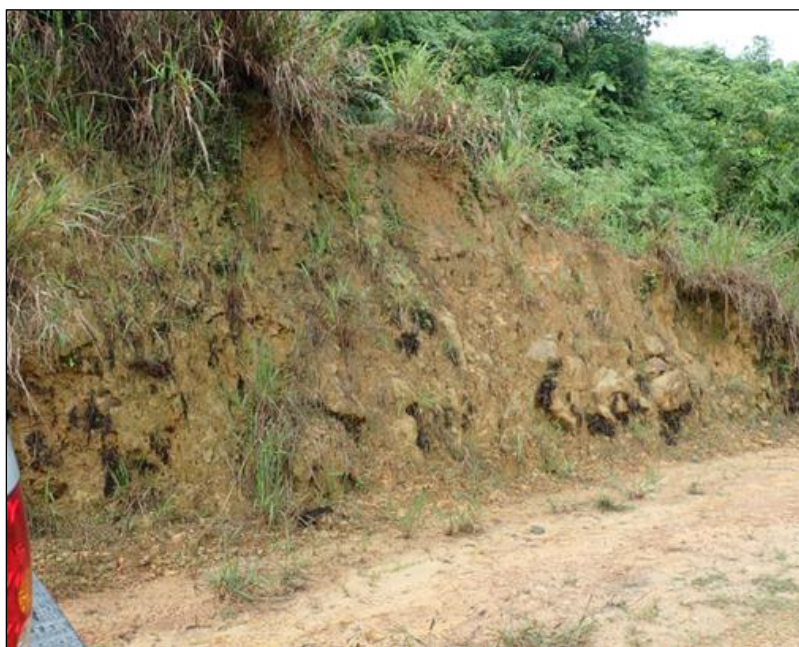
Plate 6.32: Residual soil of mainly silt and clay expose at the Project site
