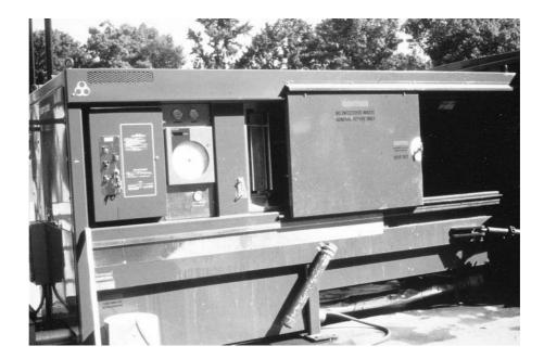
Fig. 8.8 On-site steam autoclave
