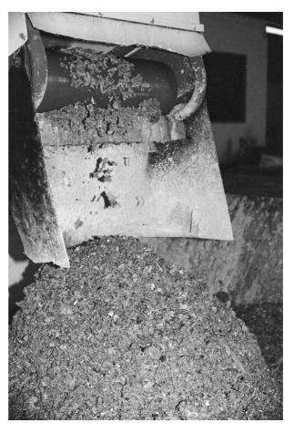
Infectious waste residues from chemical disinfection by self-contained system
