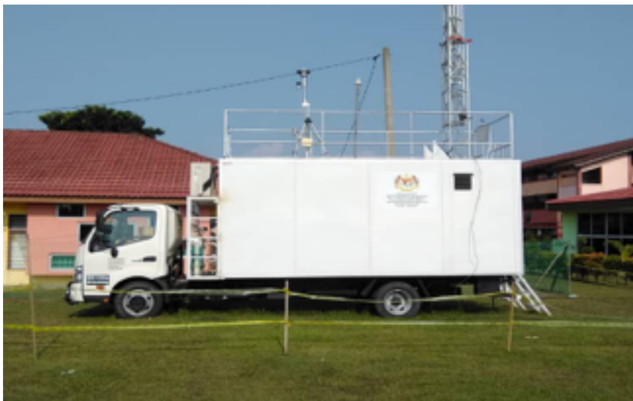
Stesen Pengawasan Kualiti Udara Bergerak Mobile Continuous Air Quality Monitoring Station (MCAQM)
